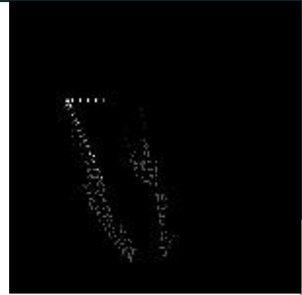
Pointcloud to grid, empty cell due to downsampling
